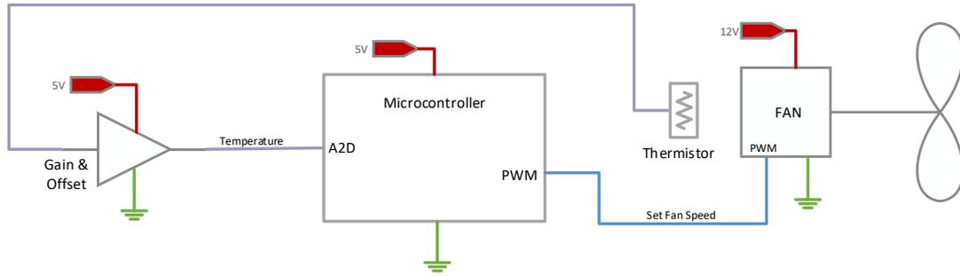
**Figure 1 – Fan Control Block Diagram**
