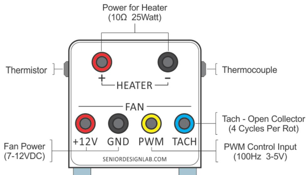
**Figure 2 – Fan Control Test Fixture**
