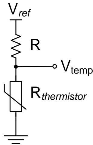
The voltage at the node  $V_{temp}$  represents the current temperature as determined by the following voltage divider equation:
