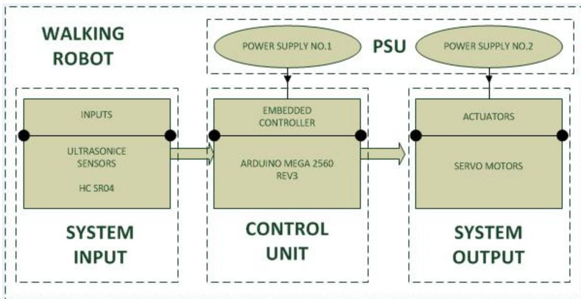
As seen, the walking robot has four main blocks:
