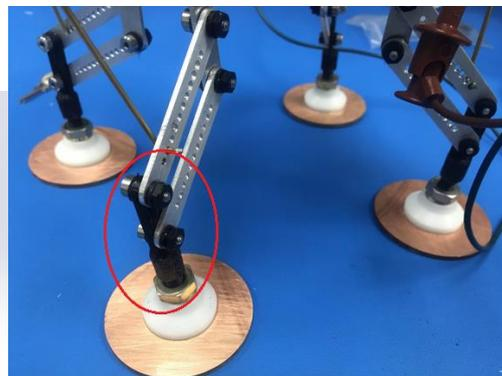
Once all of the parts of our mechanical assembly were fabricated, hardware had to be chosen that would ensure a rigidly assembled robot. To achieve this we used: Precision ground shoulder screws for all of the leg segments, rubber washers that
